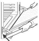
HINĞE SLOT - Door removed from the oven Figure 2
